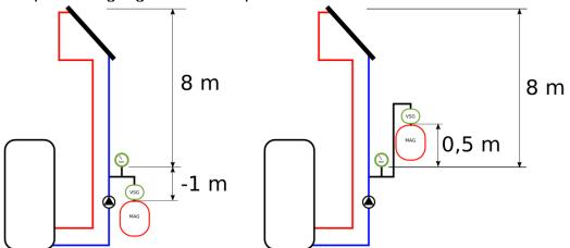
A negative height, e.g. The expansion vessel is mounted below the manometer. A positive height means the mounting of the expansion vessel above (figure to the right) of the manometer.
