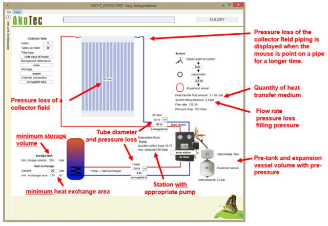
**Note**: Especially in the case of long pipelines, it may be useful to adjust the dimensions of the pipeline manually. A very high pressure loss can occur during long main strand lines.
