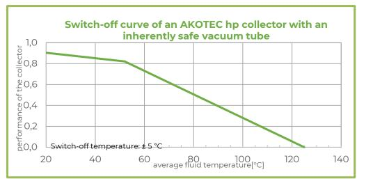
Performance tube collector at solar radiation of 1.000 W/m<sup>2</sup> (collektor with 10 tubes)
