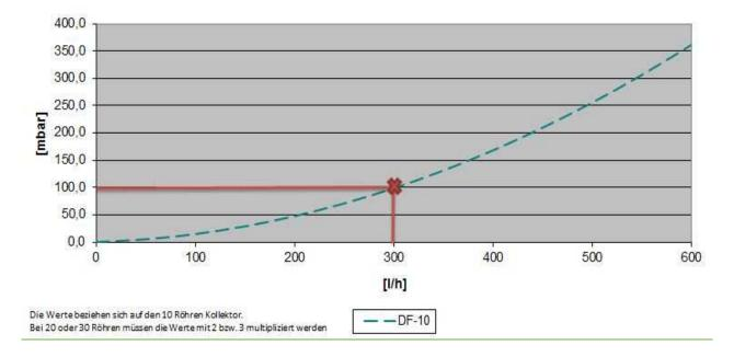
Druckverlust / pressure drop OEM Vario 1000 df & OEM Vario 800-10 df
