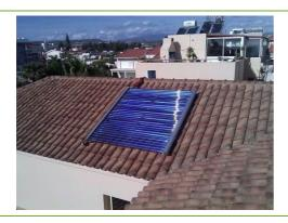
**place:** single-family house, Limasol, Zypern **plant:** 2,4 kW<sub>p</sub>, 4,8 m<sup>2</sup>, 30 direct flow Röhren **application:** domestic water heating
